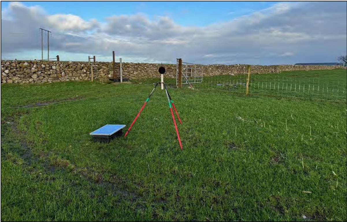
Figure 11.2: Unattended Noise Measurement Equipment
